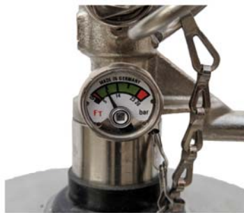
specialized pressure gauge for fire extinguisher
